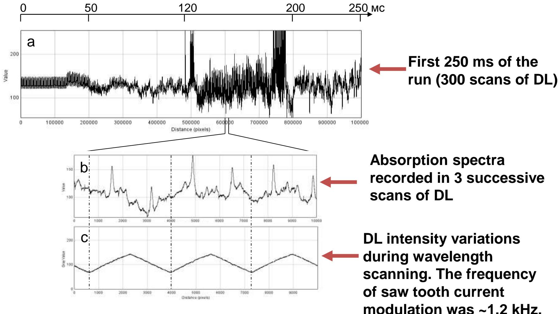
**At first step of data processing the detected transient absorption spectra were transformed into 2D image. This procedure greatly simplified the general overview of data and selection of the most important periods of process evolution.**
