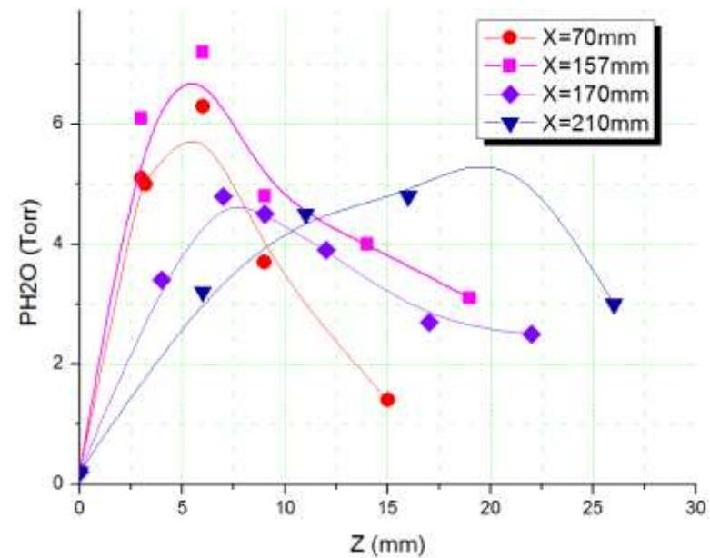
Temperature (a) and H<sub>2</sub>O vapor pressure (b) distribution measured by DLAS in plasma-assisted combustion zone for ethylene-air pair.
