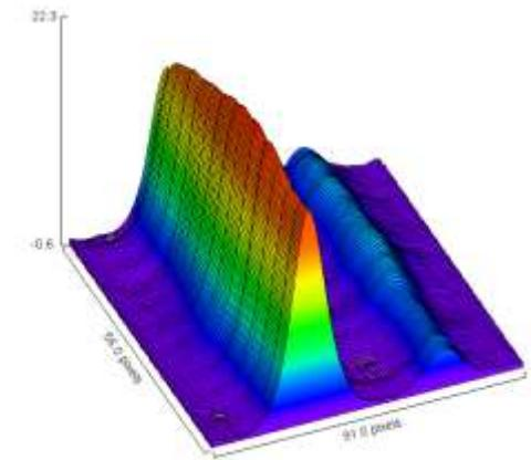
For each row in image (single TDL scan) background was constructed in the simplest way. Macros selects the first and last active points and constructs a line between them.
