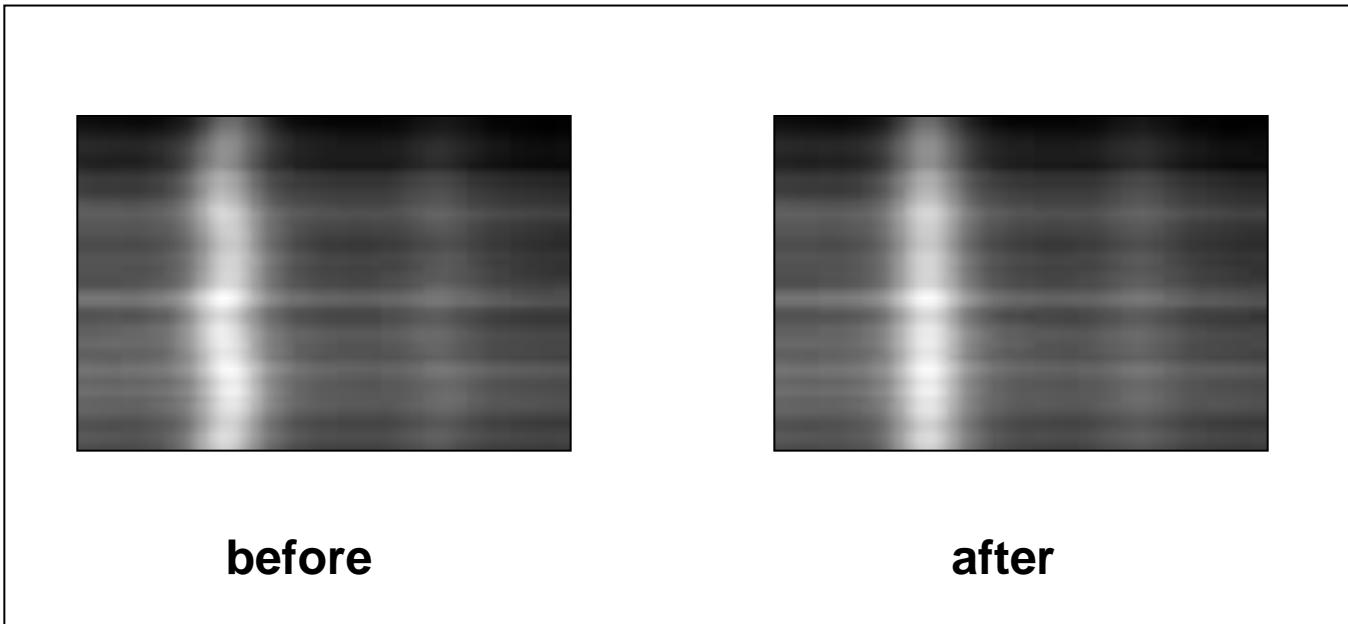
**TDL frequency jitter from scan to scan is observed in image as a light twisted line. The jitter can be removed by converting image to stack consisting of images corresponding to sequential rows and using Image Stabilizer. This plugin aligns images in stack using geometrical transformations.**
